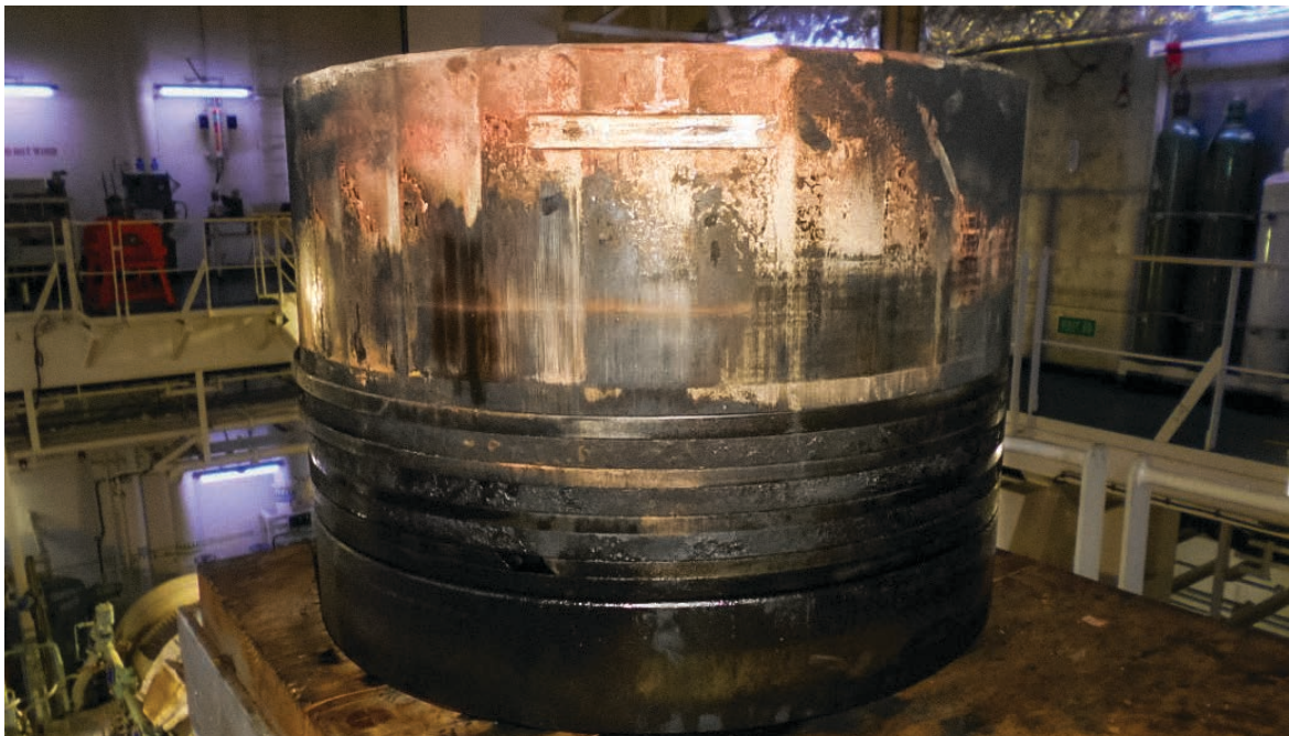
Example of a piston with scuffing and deposits. Photo courtesy of Chevron Marine Lubricants, 2020
