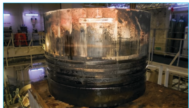
A) Piston with scuffing and deposits.
