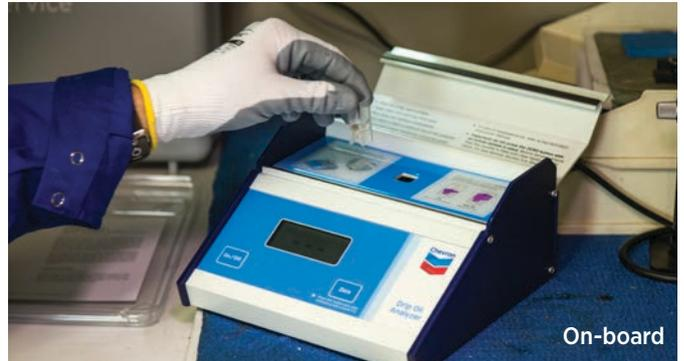
**Chevron Marine Lubricants DOT.FAST® and FAST™ services provide both on-board and on-shore analysis of drip oil, giving an accurate measurement of total iron wear, including corrosive wear.**
